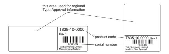
Figure 1.1 Typical Product Code & Serial Number Labels
