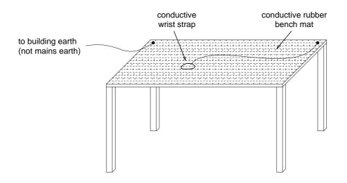
Figure 1.2 Typical Anti-static Bench Set-up
